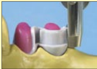
The stud-head screw is only slightly screwed into the threaded sleeve and held to the wax model using the parallel mandrel.
