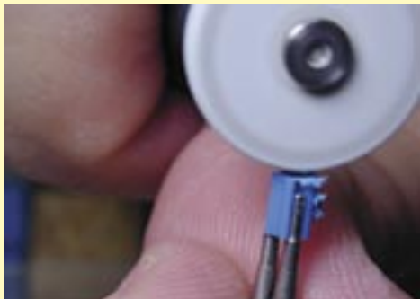
Adjust VS-3 Mini patrix from the bottom first (angled area). TIP: Use the SV Mandrel to hold the patrix while adjusting.
