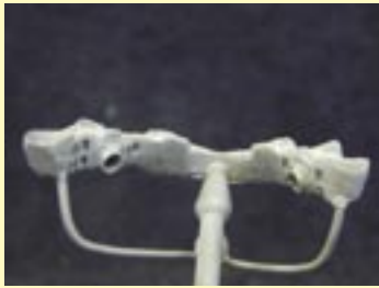
The abutments are cast, finished and milled in preparation for the overcasting fabrication.
