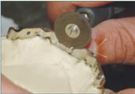
Cut off the excess screw shaft.
