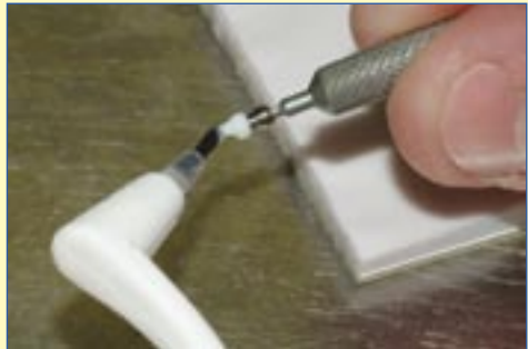
Coat the threaded portion of the ball screw with cement.
