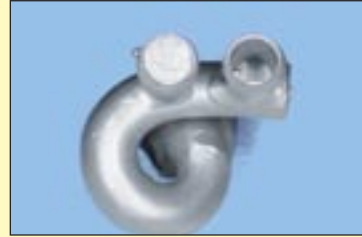
The considerable expansion of the competitor's resin during the incineration phase resulted in the fracture of the investment material die in the casting ring. After casting, the crown is sealed with a lid and cannot be used. A section through the cast crown shows the fractured die.
