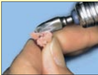
Through friction heat during grinding and high heat sensitivity, the plasticity phase of the competitor's resin can be reached. Deformation of the model, rough grinding surfaces, and inadequate fit may result.
