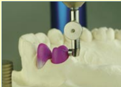
A 1.7mm auxiliary modeling element (#450 000 73) is placed into a VKS paralleling mandrel and is waxed to the coping using a surveyor. The modeling element creates a 0.5mm larger receptacle to accommodate the cement used to bond in the threaded sleeve.
