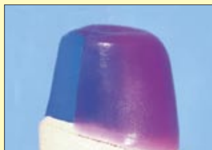
Uniform coping thickness due to perfect scraping properties. When the die shines through, a layer thickness of 0.3 to 0.4 mm has been achieved.
