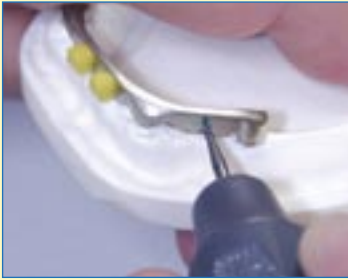
A small dimple is prepared with the Diatit Center Drill (#330 006 60) to determine the position of the drill hole. The dimple is used to guide the drill hole. The dimple will center the drill and keep it in position.
