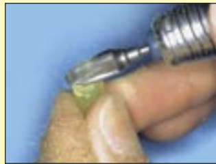
Pi-Ku-Plast features dimensional stability; during grinding fine shavings are obtained and a smooth grinding surface is ensured.
