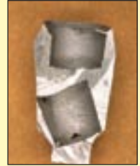
The considerable expansion of the competitor's resin during the incineration phase resulted in the fracture of the investment material die in the casting ring. After casting, the crown is sealed with a lid and cannot be used. A section through the cast crown shows the fractured die.
