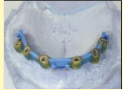
3. The implant frame is waxed up using the SG bar patrx.
