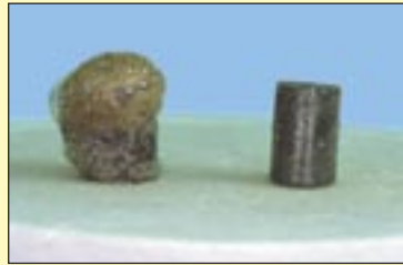
At 275°C the competitor's product foams and expands considerably.
