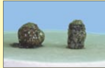
At 300°C the competitor's product reveals distinctive expansion whereas Pi-Ku-Plast reduces in volume.
