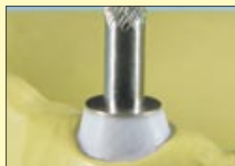
Colloidal graphite (#540 007 06) is applied onto the thread of the casting screw; then the screw is turned into the threaded sleeve exerting minimum force.
