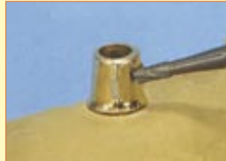
A centering drill is used to create a dimple in the correct position.
