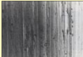
Scanning electron microscope picture of the inner side of a telescopic secondary element made of a precious metal alloy with a magnification of 100.
