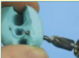
Openings (inlet & outlet) are drilled into the matrix using the locating matrix drill and Multi-Sep is applied.
