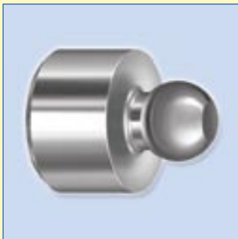
A 1.7mm auxiliary modeling element (#450 000 73) is placed into a VKS paralleling mandrel and is waxed to the coping using a surveyor. The modeling element creates a 0.5mm larger receptacle to accommodate the cement used to bond in the threaded sleeve.
