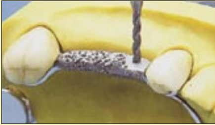
Selecting a high speed ensures safe and precise drilling even in hard CoCr alloys.
