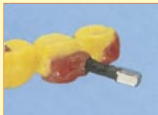
Screw a retention screw coated with colloidal graphite into the threaded sleeve to retain it in the investment material (#540 007 06).
