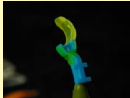
Lift off the custom, castable housing with lingual arm pattern and cast as usual.
