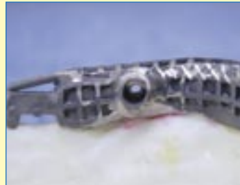
Once the overcasting is seated, the hole in the bar should be clearly visible through the housing created by the Pi-Ku-Plast around the Waxing Pin
