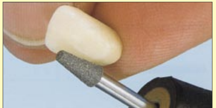
The conical grinding tool has a coated face which provides for universal application. The entire design process can be completed with this tool.
