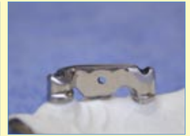
Access hole is drilled using the 1.4 mm center drill and multidrill. Milling oil is recommended.
