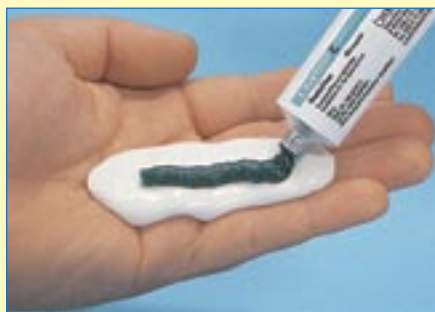
A measuring spoon of Exaktosil C kneading silicone is mixed with 3 cm of hardener paste.
