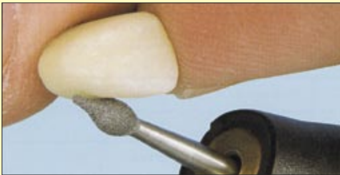
The concave part of this tool ensures perfect contouring of the approximal surfaces around the neck of the tooth. Enhanced aesthetics in less time.
