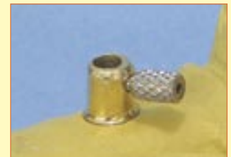
Screw the threaded rod into the sleeve. Both the pin and the hexagonal socket can be reduced as required.
