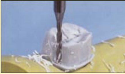
Excellent milling of wax due to the adjustable speed control.
