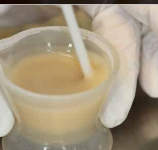
Evenly mix in top.lign professional with a mixing ratio of 10 g to 7 ml and leave to soak for 30 seconds.
